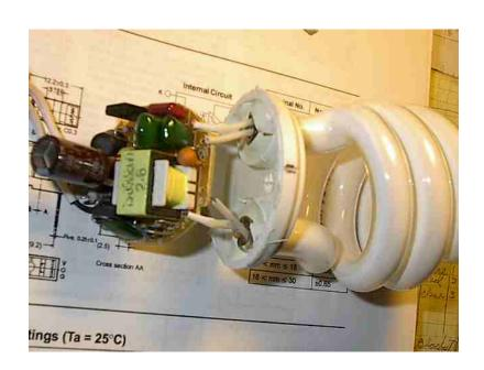
The sales pitch is that compact fluorescent lamps (CFL's) are "green" and good for you, and the planet. Well, they do use less power. But to do so, they incorporate a voltage converter as seen in the disassembly above. This emits throughout the room EMR at between 25-60KHz. Its rapid switching operations also feed electrical spikes, or "dirty electricity", into
