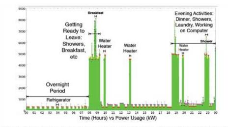
Without detailed knowledge of appliance signatures, intuitive observation with power consumption variations indicates human activity. Credit: "Private Memoirs of a Smart Meter," Molina-Markham, et.al., 2nd ACM Workshop On Embedded Sensing Systems For Energy-Efficiency In Buildings (BuildSys 2010), Zurich, Switzerland, November 2, 2010.
