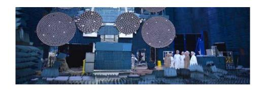
Sky Muster, first of several NBN satellites to beam down 26.5-40GHz microwaves.
