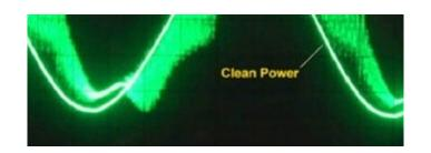
Distortion of a smoothly alternating, 50/60Hz mains current by switching spikes from a connected smart meter.
