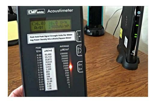
Measuring microwave radiation from a domestic wireless internet modem.
